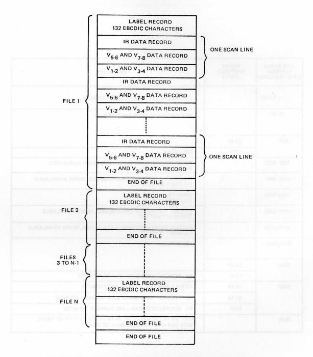
Figure B-8. Master Data and Experimenter History Tape File Format for Mode B Data
