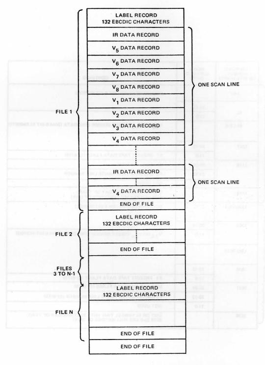
Figure B-7. Master Data and Experimenter History Tape File Format for Mode A Data
