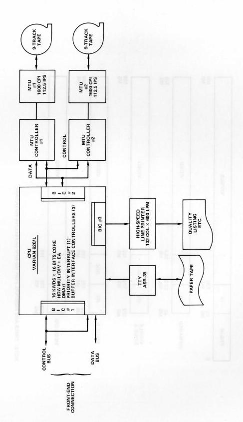
Figure 3-3. A-3 Processing System Computer Configuration
