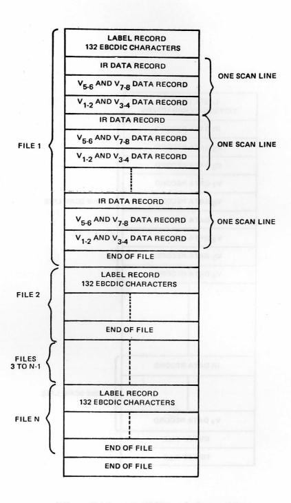
Figure B-3. VISSR Preedit Tape File Format for Mode B Data
