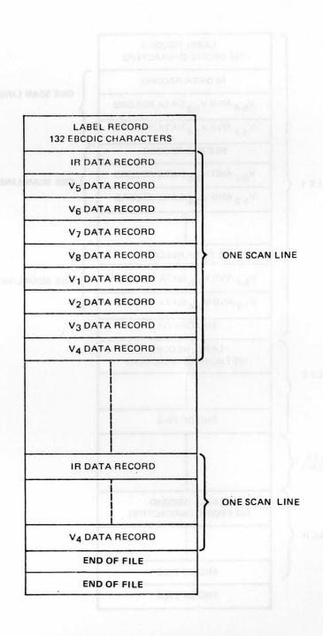
Figure B-2. VISSR Preedit Tape File Format for Mode A Data
