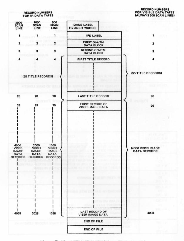
Figure B-15. VISSR IDAMS Picture Tape Format
