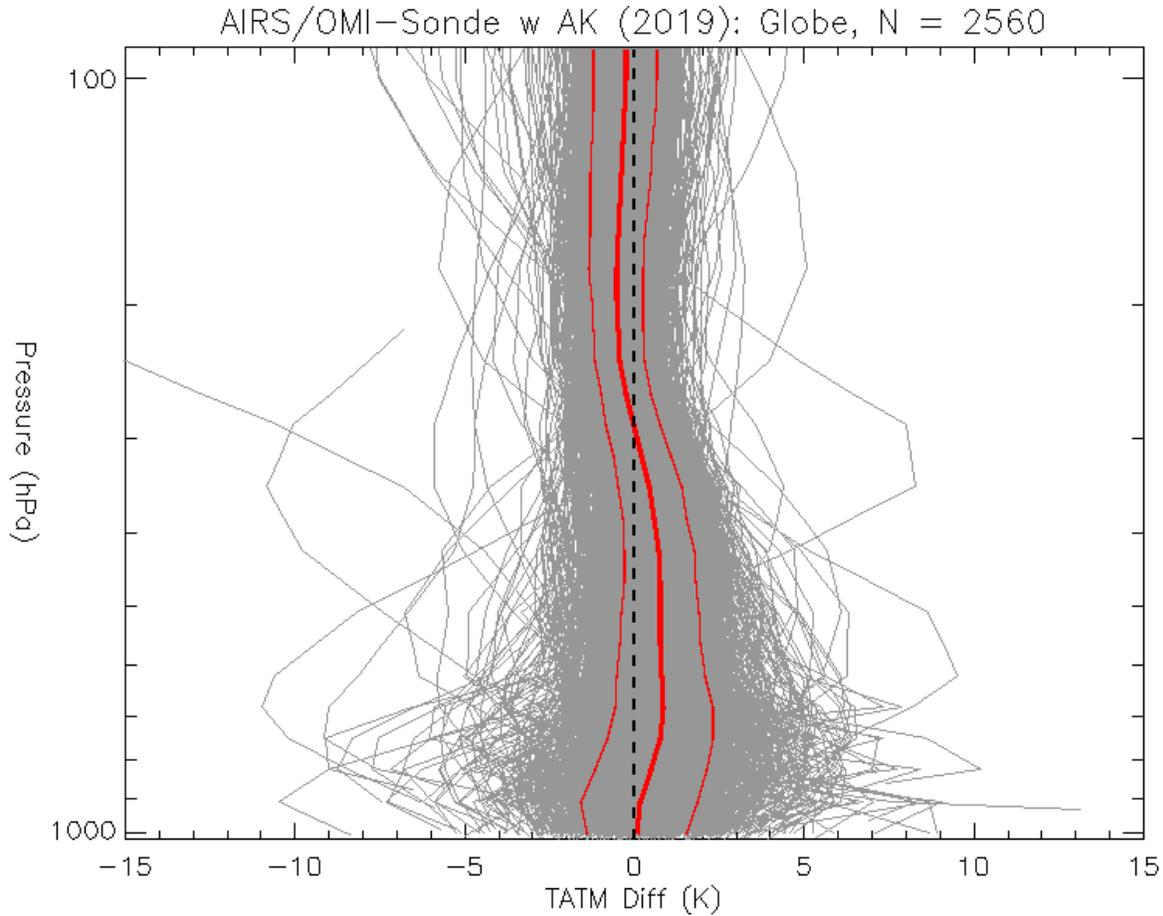
**Figure 2.** AIRS-Only TATM minus radiosonde temperature with averaging kernel applied for 2560 global matches within 50 km and +1.5 / -0.5 hours. Also shown are mean difference (thick red line) and mean $\pm$ rms (thin red lines).
